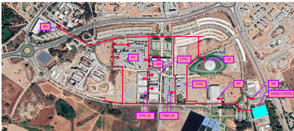
Figure 2-44. UCY_DH. University of Cyprus – District heating schematic.
